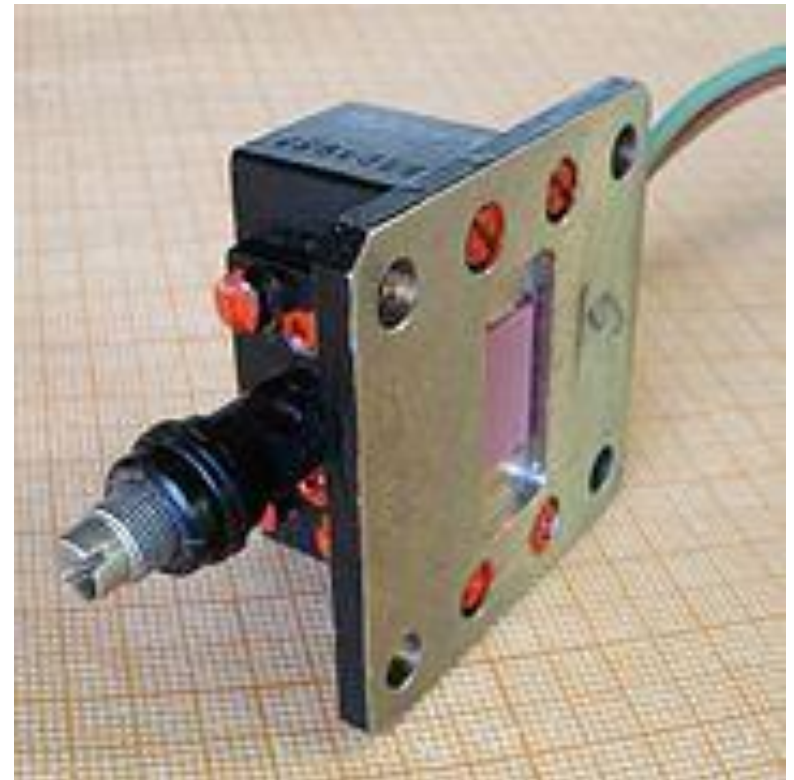
Figure 2 Coaxial Cavity Based Gunn Diode Oscillator Design
