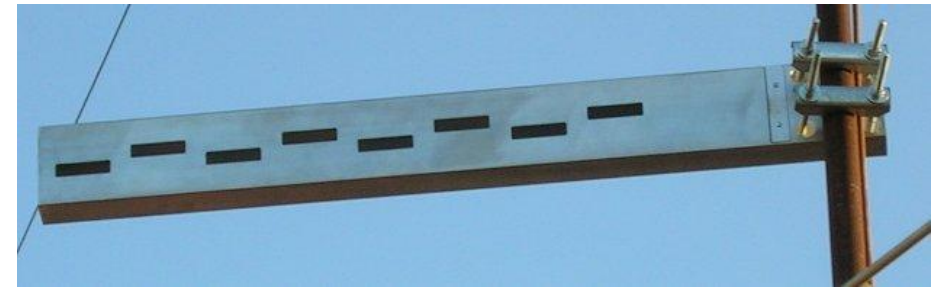
(b) Slot Antenna
